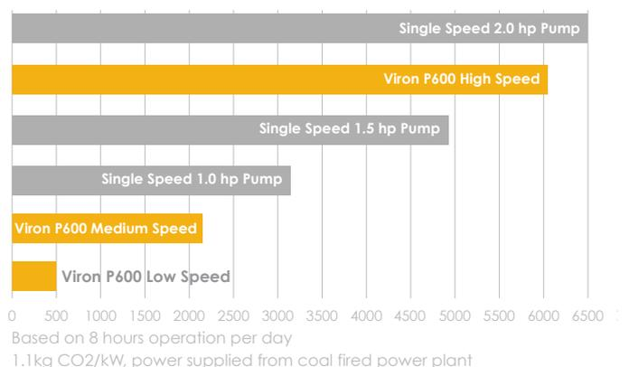
\* Annual Operating Cost based on operating pumps at factory preset low speed for 8 hours a day, each day of the year. Actual operating costs may vary according to time spent on higher speeds and the actual speed required to effectively circulate water throughout pool, filtration and plumbing system.
