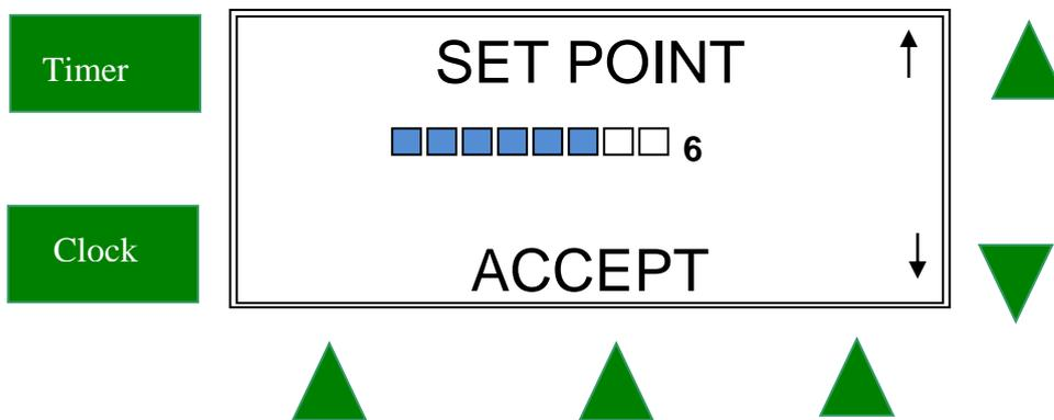
Use the up and down buttons to change the Set Point between 0 and 8. 0 chlorine output should only be used when there is no salt in the water. In summer, the chlorine should be set between 6 and 8 and you should regularly check your chlorine level in your swimming pool to determine if the output should be increased or decreased. Rely on your pool professional for advice on the recommended chlorine level in your pool.
