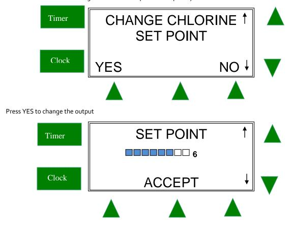
Use the up and down buttons to change the Set Point between o and 8. o chlorine output should only be used when there is no salt in the water. In summer, the chlorine should be set between 6 and 8 and you should regularly check your chlorine level in your swimming pool to determine if the output should be increased or decreased. Rely on your pool professional for advice on the recommended chlorine level in your pool.
